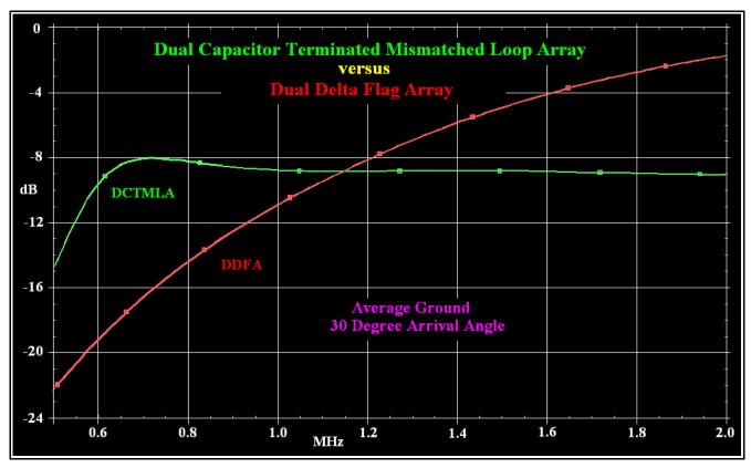
The second main reason the PSpice antenna simulation methods were developed was to model quad capacitor terminated mismatched loop arrays which also are not easily modeled with EZNEC due to their high SWR losses. Moreover, while the dual capacitor terminated mismatched loop array was easy to test in the limited space available, the quad version was not because it requires about 400' of linear space.
