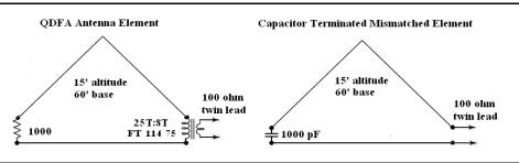
1000 pF capacitors, and delete the antenna transformers and connect the 100 ohm twin leads directly to the loop elements. For detailed information about the QDFA see "Phased Delta Flag Arrays."
