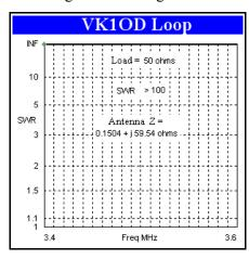
the SWR loss accounts for the difference of about 19 dB between the EZNEC simulation value and the PSpice value and antenna factor value. In general, EZNEC does not seem to provide a way to adjust for SWR loss when the SWR value is extremely high. Only when the SWR is near 1:1 is it easy to correct for; no SWR correction is required in that case.
