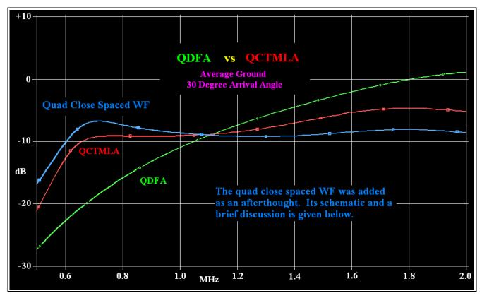
The only difference between the QDFA and the capacitor terminated mismatched version is the antenna elements, shown at right. It is trivial to convert a QFDFA to a capacitor terminated mismatched version. Replace the resistors with
