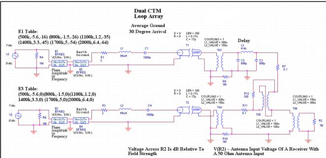
The following figure is a comparison of the dual delta flag array and the dual capacitor terminated mismatched loop array for average ground and 30 degree arrival angle. For an account of the discovery of dual capacitor
