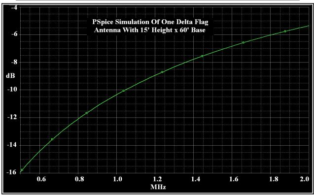
The simulation agrees with EZNEC to within 1 dB, assuming that the single flag antenna which EZNEC models is impedance matched to the receiver (which can easily be done with a broadband transformer). The PSpice schematic already includes impedance matching. This may be regarded as establishing the validity of the PSpice antenna simulation method for average ground and arrival angles in the neighborhood of 30 degrees.
